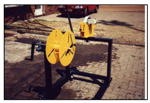
The mobile coiler was designed to accommodate the need in the wholesale and retail industry where coiling from a racking and shelving system is required. As space is limited in aisles the frame is fitted with braked castors to allow for easy maneuverability in the workplace. When required the mobile coiler is moved to the shelving system, cable is measured, coiled and cut. Once the operation is complete the unit is simply moved out of the way.
